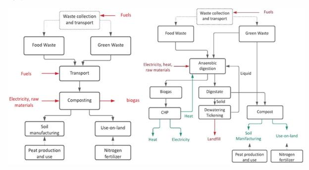
Figure 13 – System boundaries for Scenario C – Incineration (left) and Scenario D – Anaerobic Digestion and Composting (right)
