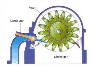
*Figure 2 – Pelton turbine installed in mini-hydropower station* [3]
