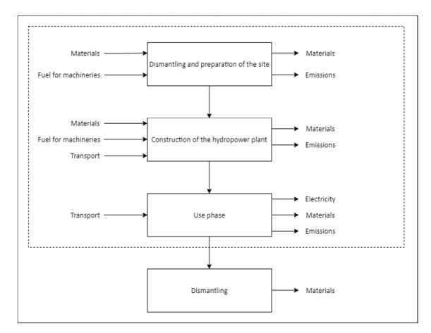
*Figure 8 – Mini –hydropower plant System boundaries. The dotted line represents the stages included in the model*
