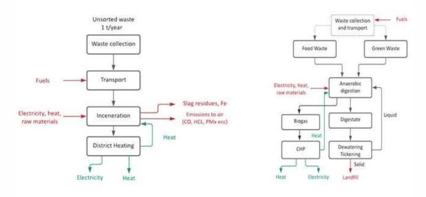
*Figure 12 – System boundaries for scenario A – Incineration (left) and scenario B – Anaerobic digestion (right)*
