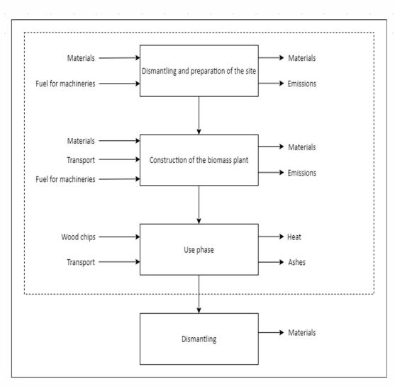
*Figure 10 – Biomass boiler system boundaries. The dotted line represents stages included in the model*
