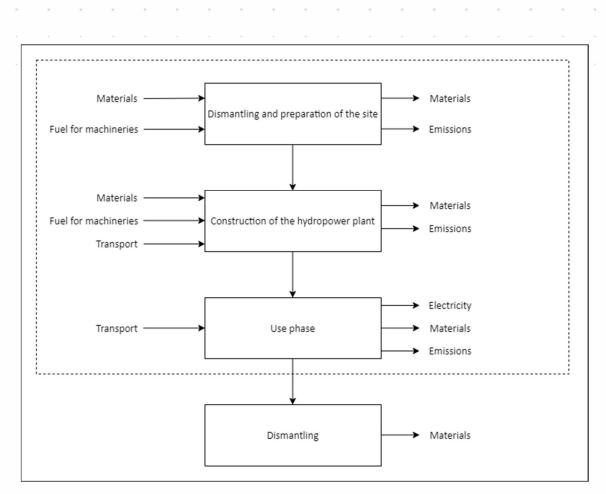
*Figure 9 – Mini –hydropower plant system boundaries. The dotted line represents stages that were included in the model*
